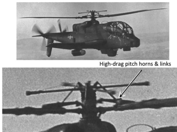
Figure 22. Lockheed AH-56A Cheyenne rotor hub showing pitch horns and pitch links contributing to high drag.
