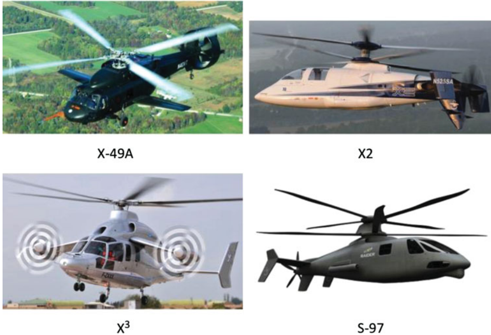
Figure 4. Newer compounds – Piasecki X-49A, Sikorsky X2, Airbus Helicopters X 3 , and Sikorsky S-97.
