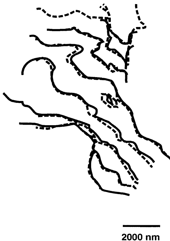
Figure 3. Tracing of features in Figure 2b and 2c, showing pit growth and retreat of steps. What appears to be a slight step growth near the edges of the figure probably is due to image drift rather than actual growth.
