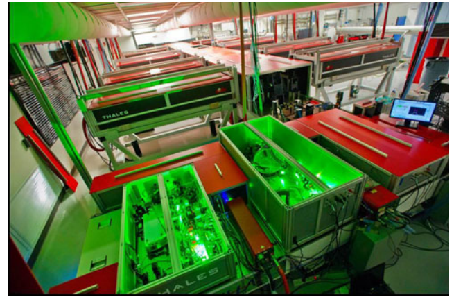
Figure 10. BELLA, the highest repetition rate petawatt class laser in the world (picture courtesy of Lawrence Berkeley National Laboratory).
