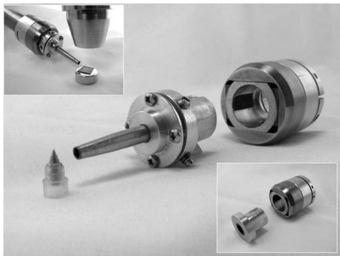
Fig. 1. Parts of the Low Energy EDS Optic. L. to R. Removable pointer for alignment, gimbaling optic assembly that fits into the electron trap, and the electron trap. Top left inset shows how the optic is used. Bottom right inset shows the electron trap with the conventional graphite collimator.
