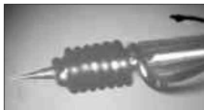
Figure. The micro-manipulator (microcoil and microtip), which measures 1 \text{mm}^3 in size, offers an alternative to the optical tweezers method. The micron-scale coil diameter and ferromagnetic tip allow these electromagnetic tweezers to be fabricated with dimensions that are much smaller than traditional magnetic tweezers.
