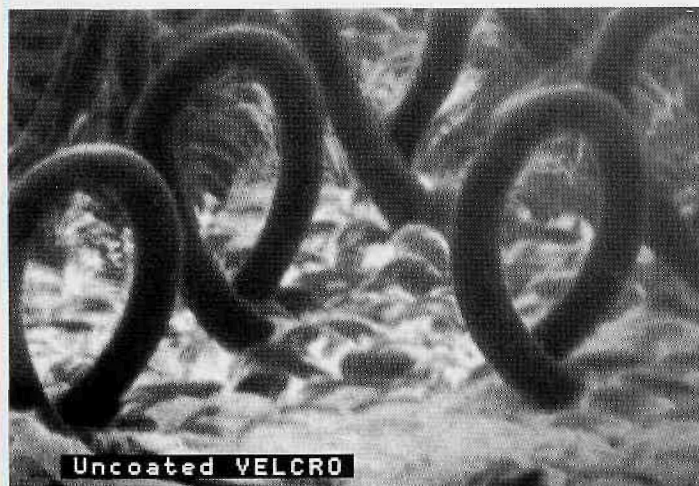
Figure 1. a) Ultra low accelerating voltage image of an uncoated Velcro sample taken with 100 eV accelerating voltage in 1987 with an SEM equipped with a lanthanum hexaboride electron source.
