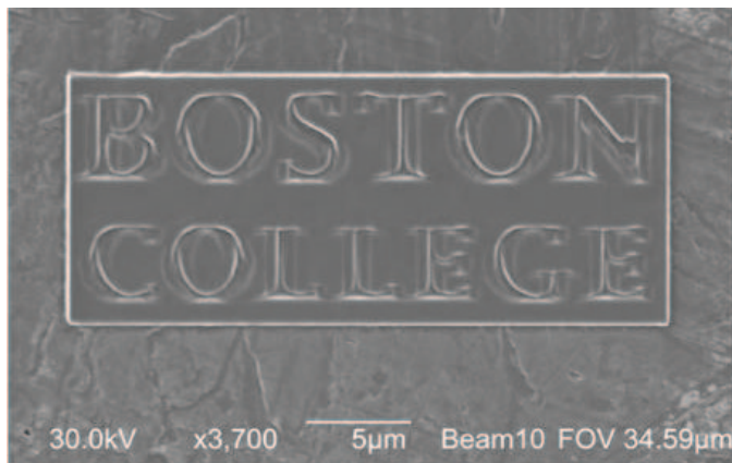
Figure 10: Negative FIB carbon deposit of the Boston College logo.
