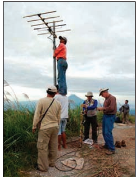
Figure 25.6 VDAP and CVGHM scientists install a seismic station to monitor volcanic activity in North Sulawesi. USGS photo.
