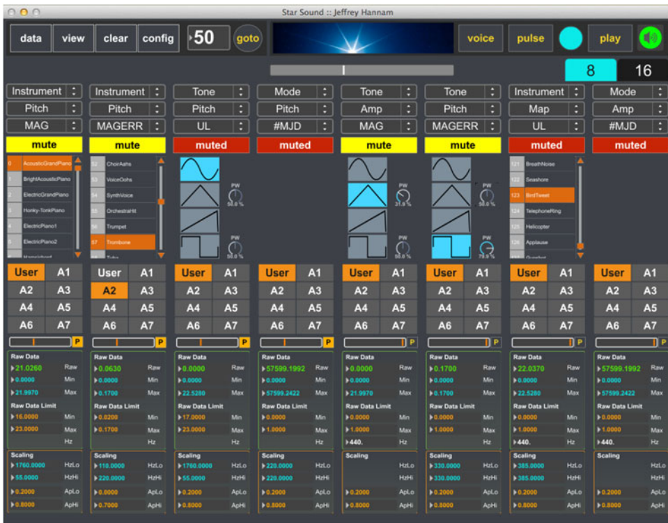
Figure 1. Image of the StarSound graphical user interface in an example configuration. Across the top, from left to right, the interface offers the following menu options; loading a data set, viewing and clearing a data set, and loading a configuration file. Below that is the scanning slider and two tabs for switching between the 16 available sonification modules. Each sonification module consists of a tone generator or musical instrument selection. A predefined pitch table is provided for mapping and listening to data quickly. From there, users may wish to fine-tune or define their own pitch range. Once a data and configuration file is loaded, the Play feature can be used to listen to the results of the data sonification from start to finish. Alternatively, the GoTo option can be used to jump directly to a point of interest, or the user can scan the data manually with the left/right keys on a computer keyboard or the scanning slider, which can be mapped directly to a stereo panning algorithm including external mouse or trackpad input. Further options include turning on the Voice accessibility for reporting the sonified data index – a pulsing option which acts like a metronome for repeated listening.
