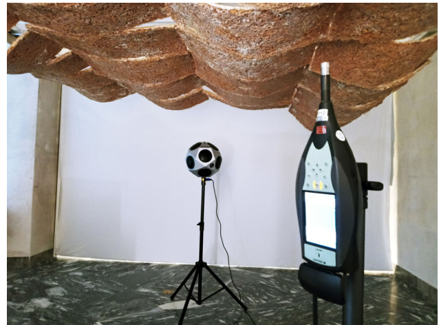
Figure 6. Acoustic test signals being played from an omnidirectional loudspeaker under the sail, and measured using a Class 1 (IEC 61672-1) laboratory-grade sound level meter, Source: Albert Dwan (Arup).
