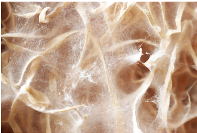
Figure 8. Detail of the composite material and the fine mycelium web after hydration, Source: Jonas Edvard.
