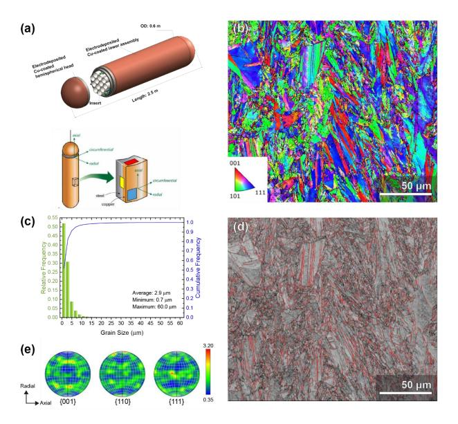
**Figure 1.** (a) Schematic diagram of the UFC and the coordinate system for characterization. (b-d) Microstructure characterizations of acid ED Cu in the circumferential direction. (b) Inverse pole figure map, (c) grain size distribution based on fitted ellipse diameter method, (d) CSL boundaries overlayed on band contrast map, (e) {001}, {110}, and {111} pole figure.
