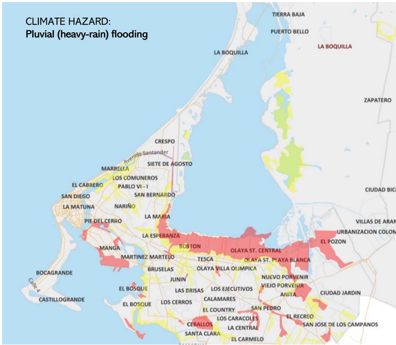
Figure 3. Risk map of pluvial flooding (due to heavy rain) with most severe impacts in the poor neighborhoods near the swamp of La Virgen. (Created with https://midas.cartagena.gov.co/ )
