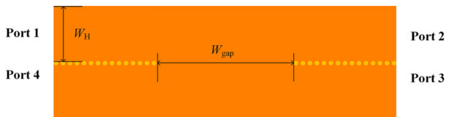
Fig. 1. Schematic of half mode substrate integrated waveguide coupler.
