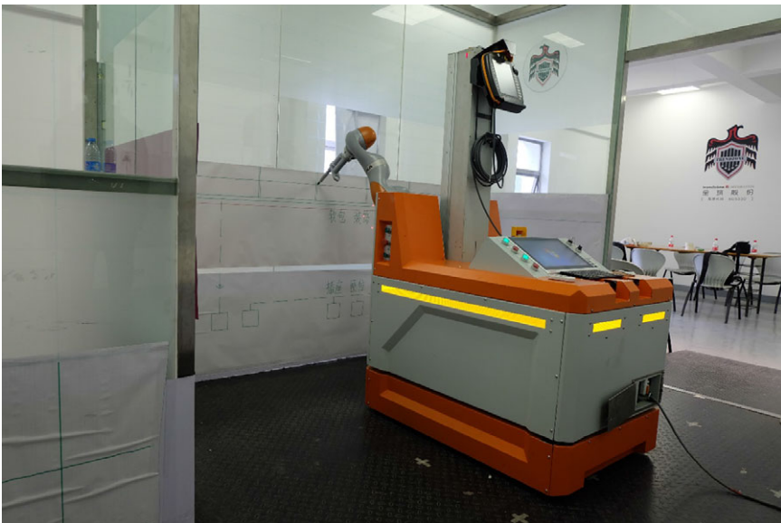
Figure 7. Baseline drawing with mobile manipulator for interior decoration.
