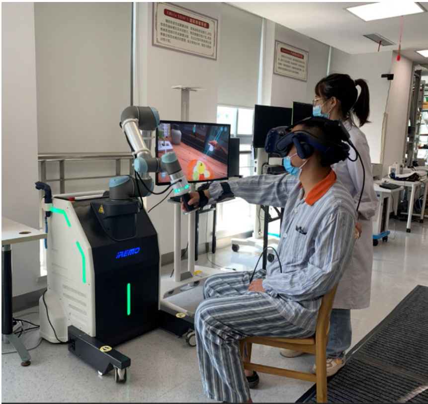
Figure 9. Upper limb rehabilitation with mobile manipulator.
