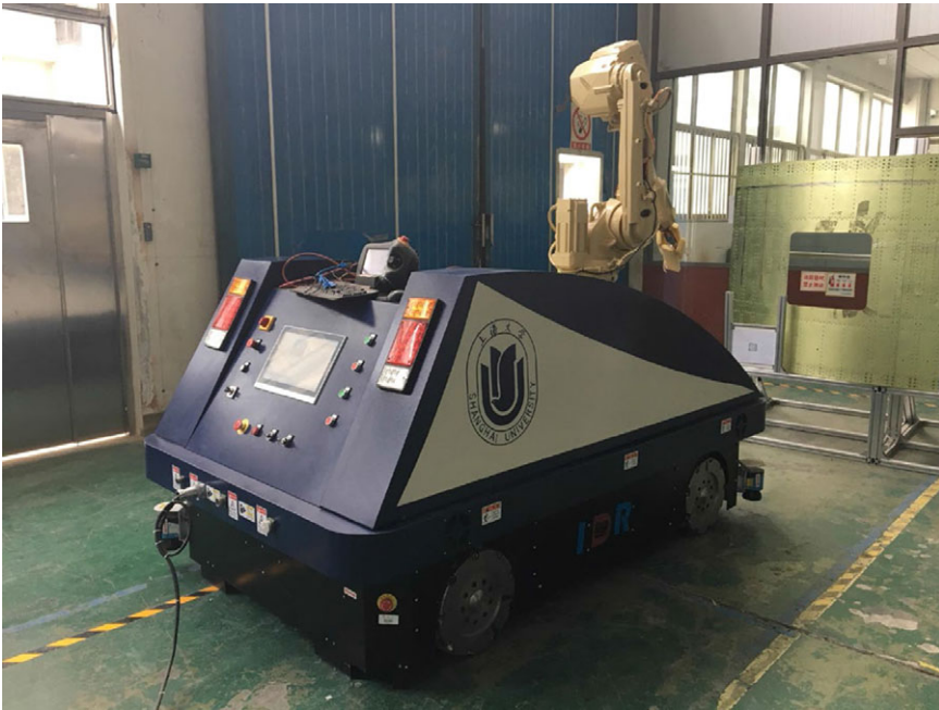
Figure 6. Fuselage drilling or riveting with mobile manipulator for aircraft manufacturing.
