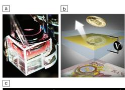
(a) Experimental setup for generating a liquid window-mirror. (b) Schematic showing the setup with a coin facing the liquid mirror and a currency note at the back of the mirror. (c) Real images observed during the transition between a transmissive "window" state (when no nanoparticles are at the interface) to a reflective "mirror" state (when nanoparticles assemble densely at the interface). Credit: Nature Materials.
