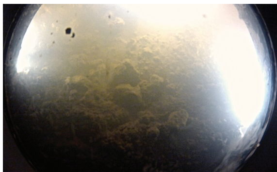
Fig. 3. Image of sediments at the bottom of SLW obtained by the MSLED camera. The top of the sedimentary layer crumbled as the camera housing touched it. The view shown here is nearly vertically down and the housing window is \sim 0.3 m in diameter.
