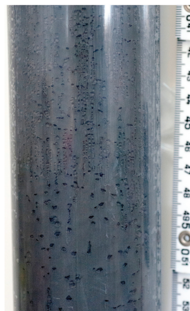
Fig. 6. Multi-corer sediment core in a transparent liner with a ruler in centimeters on the right-hand side. The dark spots are interpreted as gas bubbles formed as a result of core depressurization as it is brought up to the surface (Tulaczyk and others, 2001).
