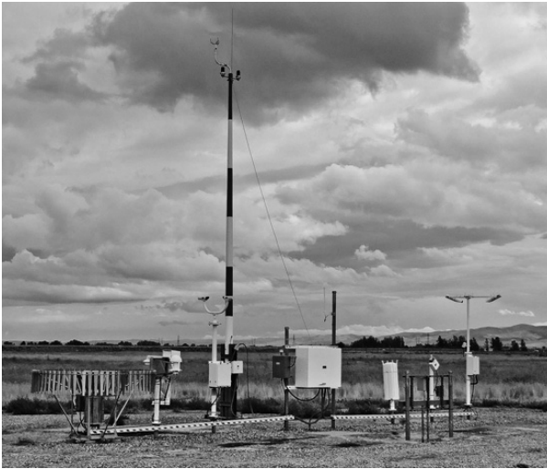
Figure 1.2 The US National Weather Service Automated Surface Observing System (ASOS) sensor package located at Pocatello, Idaho (42.917°N, 112.567°W, 1356 m above MSL, WMO station no. 72578). From left to right, the instruments shown are – heated tipping-bucket raingauge (TBR) within wind shield: aspirated temperature and humidity sensors: present weather sensor: 10 m wind mast with heated ultrasonic wind sensor: data collection panel (big box): laser ceilometers: freezing precipitation sensor (little tilted box), and finally the visibility sensor. See also www.weather.gov/asos . (Photograph by Gary Wicklund)
