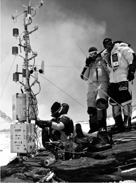
Figure 1.1 Installing one of the world's highest weather stations, the 'Balcony Station' at 8430 m above sea level on the south col of Mt Everest, just below the summit at 8849 m. (Photograph courtesy of the Ev-K2-CNR Committee archive)
