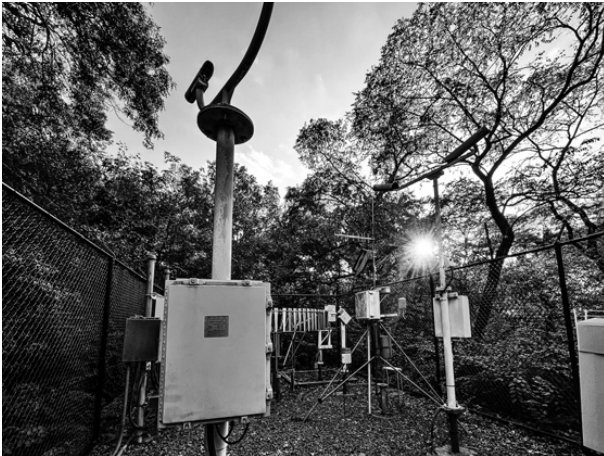
Figure 1.18 The Automated Surface Observing Site (ASOS) weather station in New York's Central Park (photograph by Simon Lee, Columbia University).
