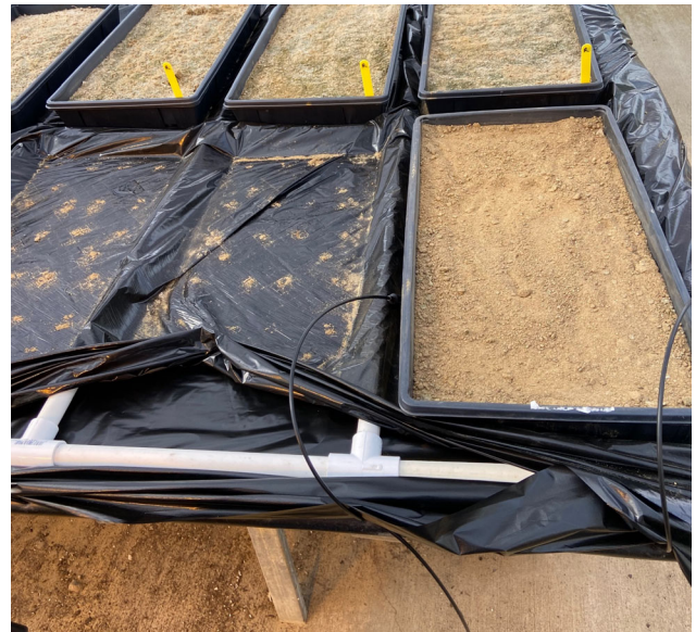
Figure 2. Greenhouse design for preemergence dose-response screening studies. Each flat filled with soil was placed in an individual cell for subirrigation to prevent herbicide contamination between flats from water movement.
