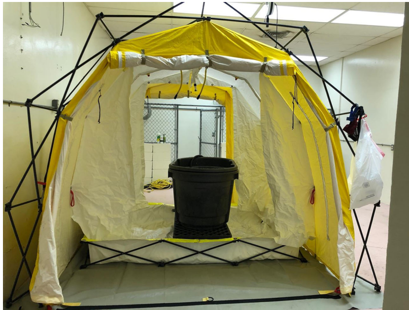
Figure 3. Example of Decon Tub System and Tent (barrier) set up.
