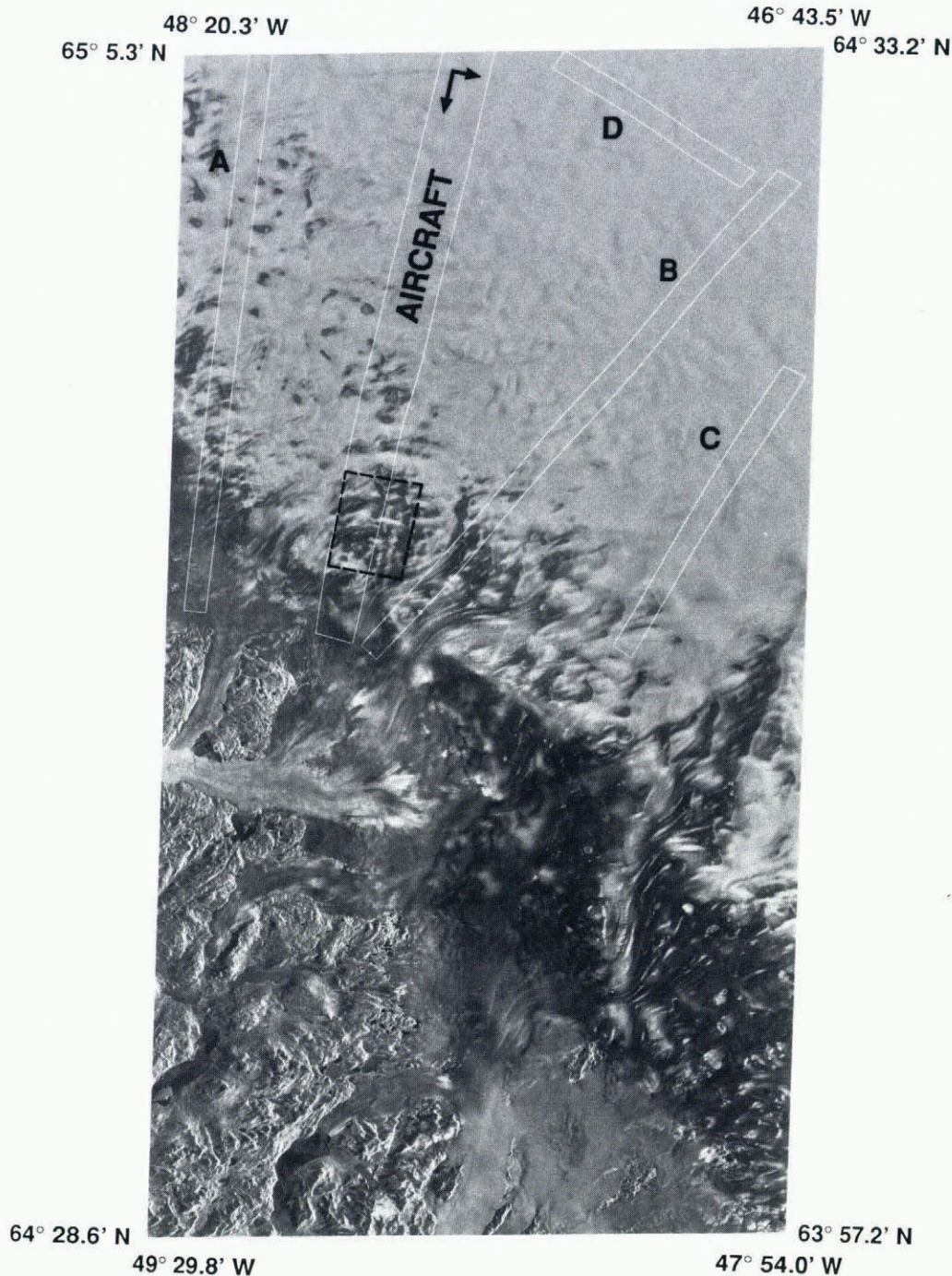
Fig. 6. Co-registered L-band SEASAT and multi-frequency aircraft SAR swaths indicating locations of the aircraft SAR track (AIRCRAFT) and other samples of data (A–D) discussed in section 6. The flight and radar-look directions are indicated by the arrows for the strip of aircraft SAR survey-processed data. The black dashed rectangular box shows the location of the full-resolution image presented in Figure 5.
