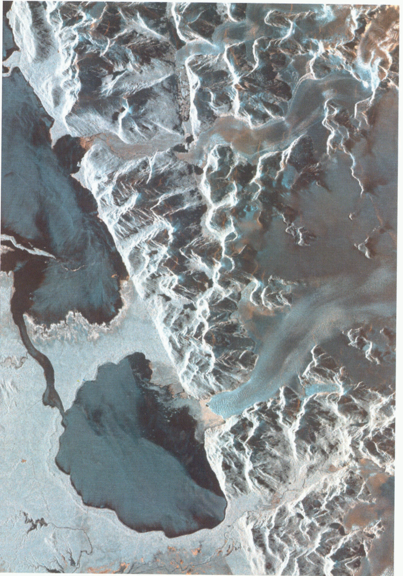
Fig. 2. False-color composite image of Glaciar San Rafael acquired by SIR-C SAR on 10 October 1994. C-band is red, C-band + L-band is green and L-band is blue.
