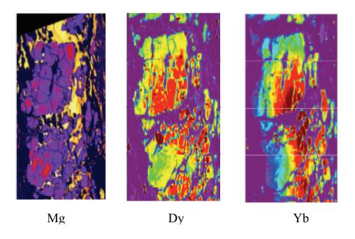
**Figure 1:** Elemental distribution of major and trace elements of an almandine garnet comparing Mg Ka (EPMA) with <sup>163</sup>Dy and <sup>172</sup>Yb (LAICPMS).
