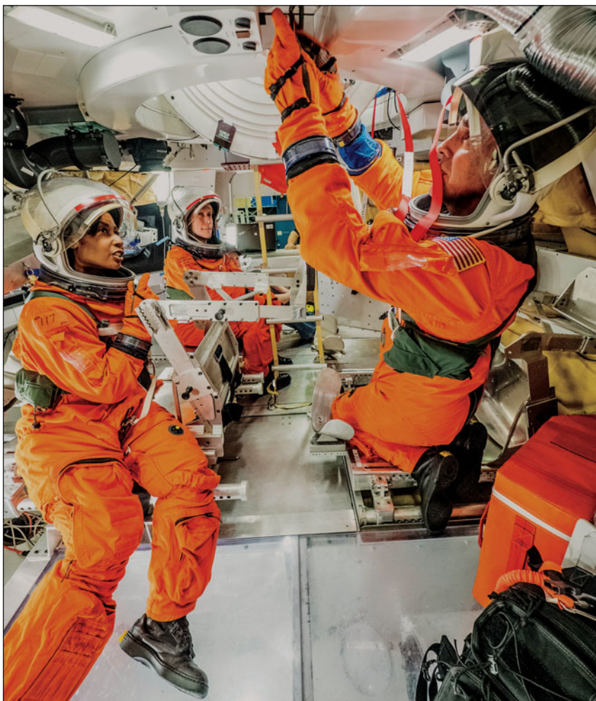
Engineers and astronauts conducted testing in a representative model of the Orion spacecraft at NASA Johnson Space Center in Houston to gather the crew’s feedback on the design of the docking hatch and on postlanding equipment operations. NASA’s goal is for Orion to carry the first human explorers to Mars. Credit: NASA.
