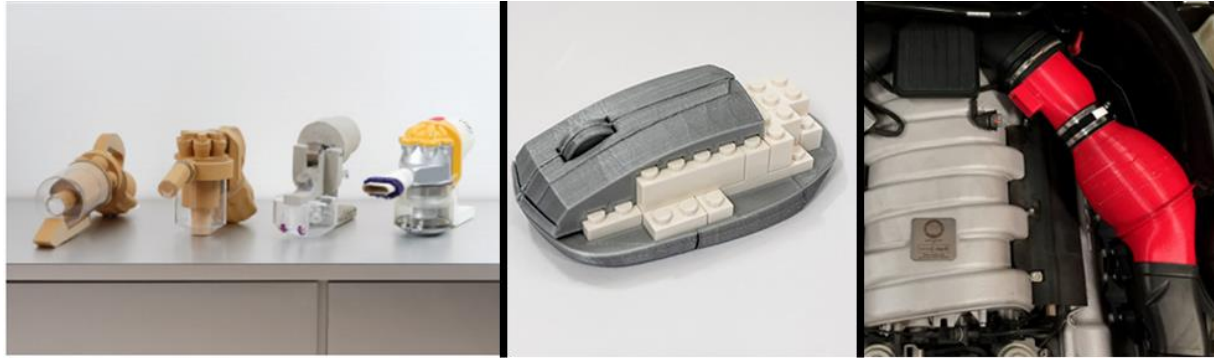
Figure 2. Examples of different prototyping methods; cardboard (James Dyson Foundation, 2019), construction kit (Mathias, 2018) and MEX (Ultimaker, 2019)
