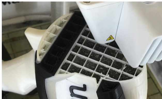
Figure 3. Design 3 being manufactured, showing the addition of mass
