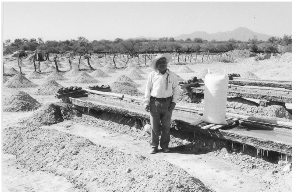
Figure 3. A finca usually has several canoas to evaporate brine under the sun. In some cases, a canoas may be up to 150 years old. Photograph by the author.
