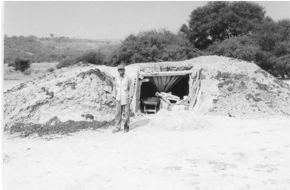
Figure 2. The leached soil is thrown to the sides of the estiladera , where it accumulates over time, forming the turrero or mound. Photograph by the author.
