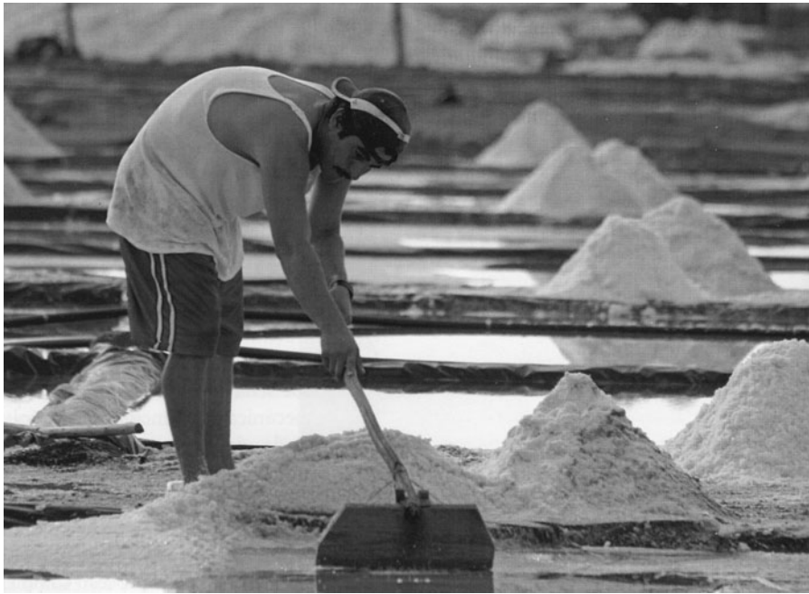
Figure 13. Crystallized salt in the era is collected with a rastrillo in Cuyutlán, Colima. Courtesy of Blas Castellón.
