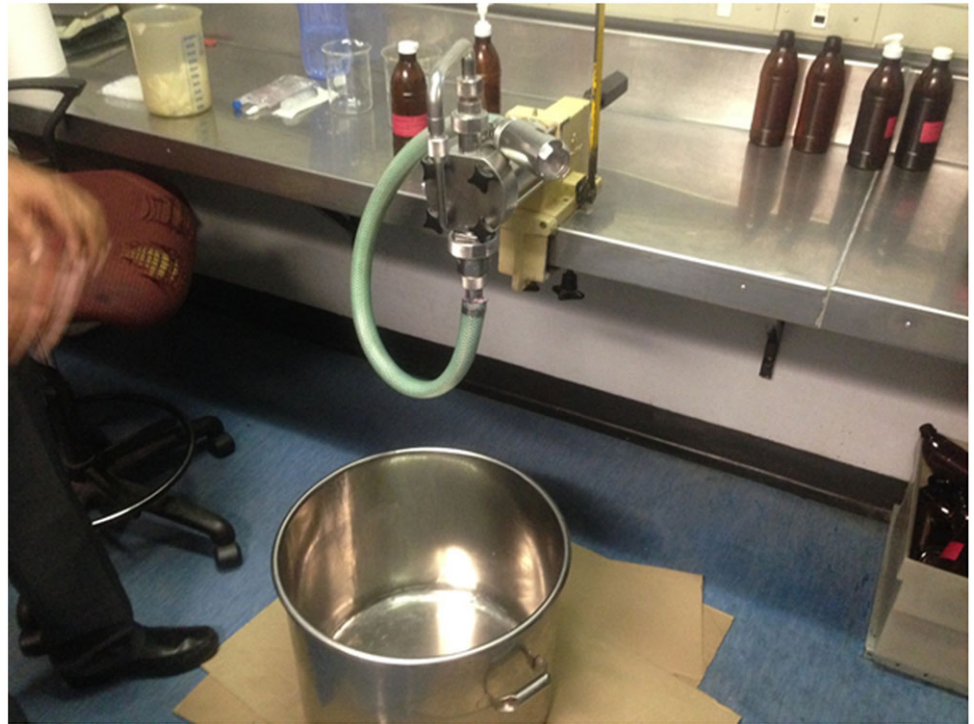
Fig. 1. The dispenser device used by the pharmacy to prepare the chlorhexidine and water solution. The chlorhexidine, water and bromothymol blue mixture are placed in the bucket on the floor, then siphoned up by the hose and filled into empty bottles which are placed beneath the nozzle.
