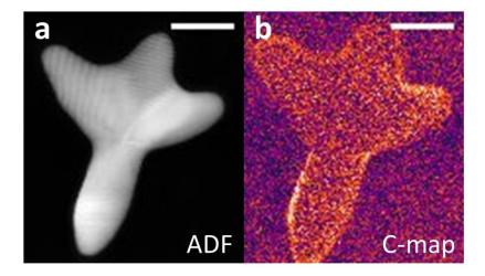
Figure 1. (a) ADF-STEM image of a single CpG conjugated gold nanostar deposited on a graphene support. (b) EELS spectral map of carbon from the same region. A carbon shell corresponding to the DNA is visible at the surface of the particle. Scale bars are 20 nm.
