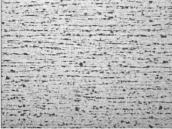
FIG. 1. Pipeline base metal. Presence of ferrite and aligned pearlite colonies. 25X.
