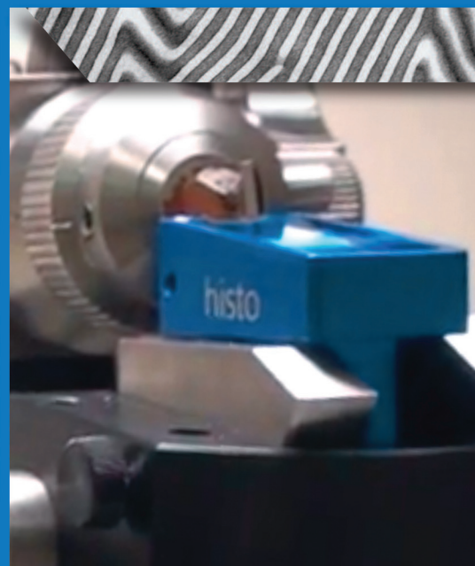
Shown: DiATOME Histo Diamond Knife producing thick sections
