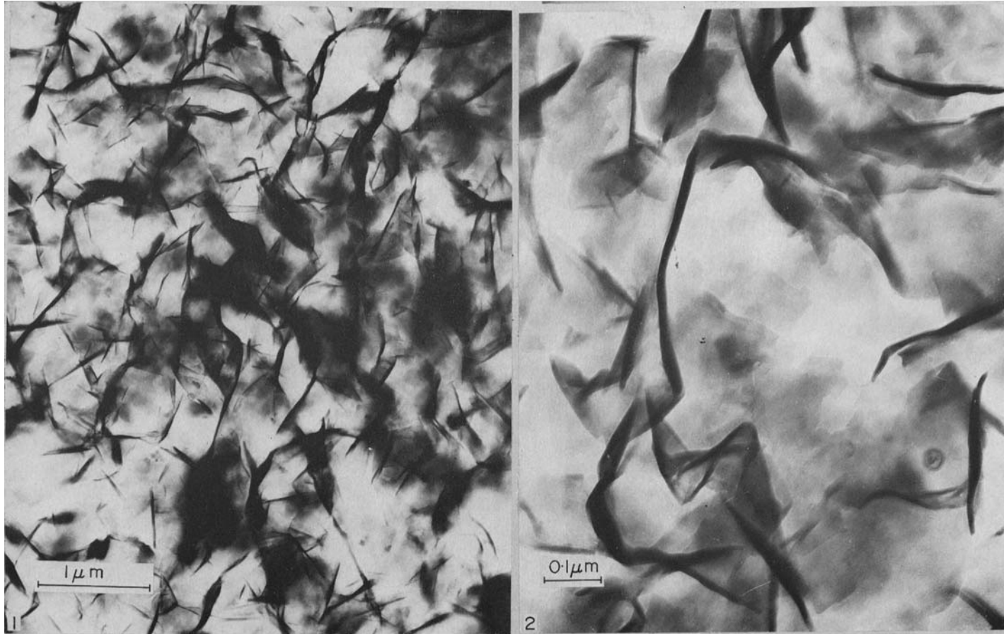
Fig. 1. Electron photomicrograph of dimethyldioctadecylammonium-montmorillonite dispersed ultrasonically and critical point dried, 41,200 \times .
