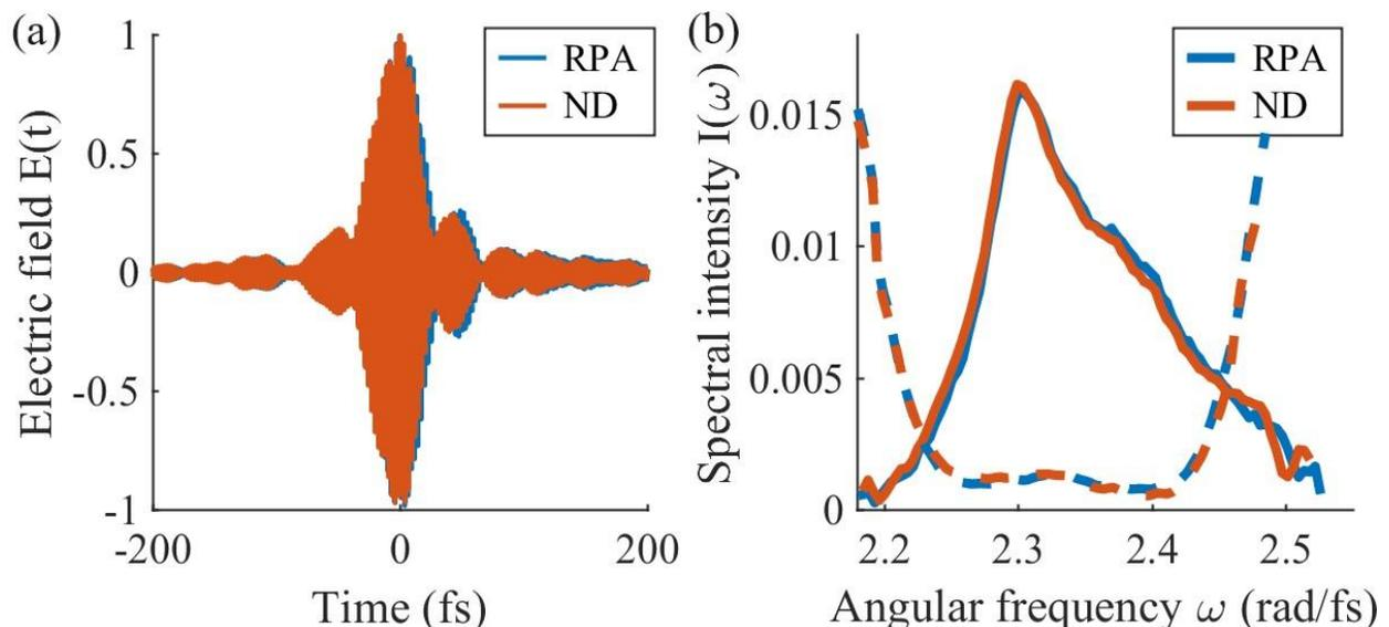
Fig. 6. Comparison of temporal characteristics of two attenuation cases. (a) Laser electric fields obtained with a ND filter (blue line) and with a RPA (red line). (b) Spectral intensities and phases of the two cases.
