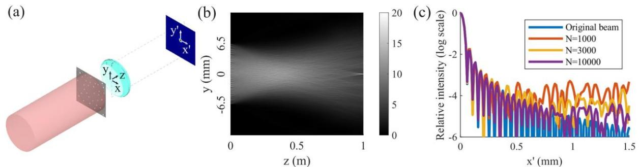
Fig. 1. Attenuation of laser intensity using a random pinhole attenuator (RPA). (a) The schematic diagram for attenuating the laser intensity using the RPA. (b) The intensity of the laser beam on the  $yz$ -plane shown in (a). (c) Intensity distribution at the focal plane calculated for different number of pinholes.
