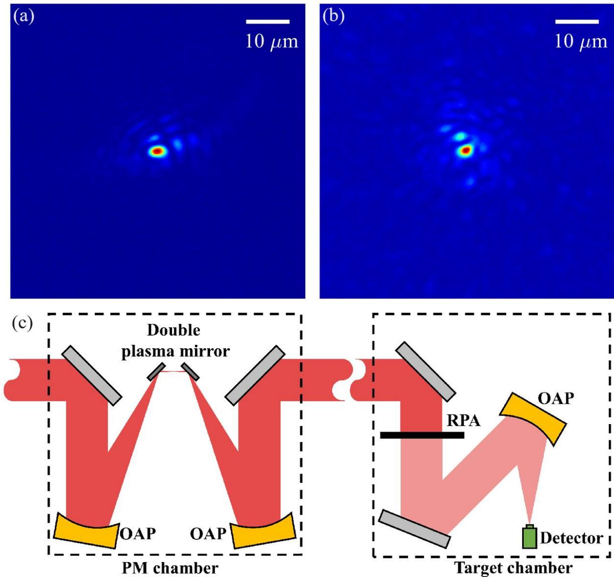
Fig. 5. Beam profiles of the CoReLS 4-PW laser. (a) Beam profile of the focused 10- $\mu$ J laser beam without passing through the plasma mirror system, and (b) Beam profile of the focused laser beam obtained with the plasma mirror system. The energy of the laser beam was 80 J before the grating pulse compressor. (c) The schematics of the CoReLS 4-PW laser. The plasma mirrors (PM), RPA, and off axis parabola (OAP) are shown.
