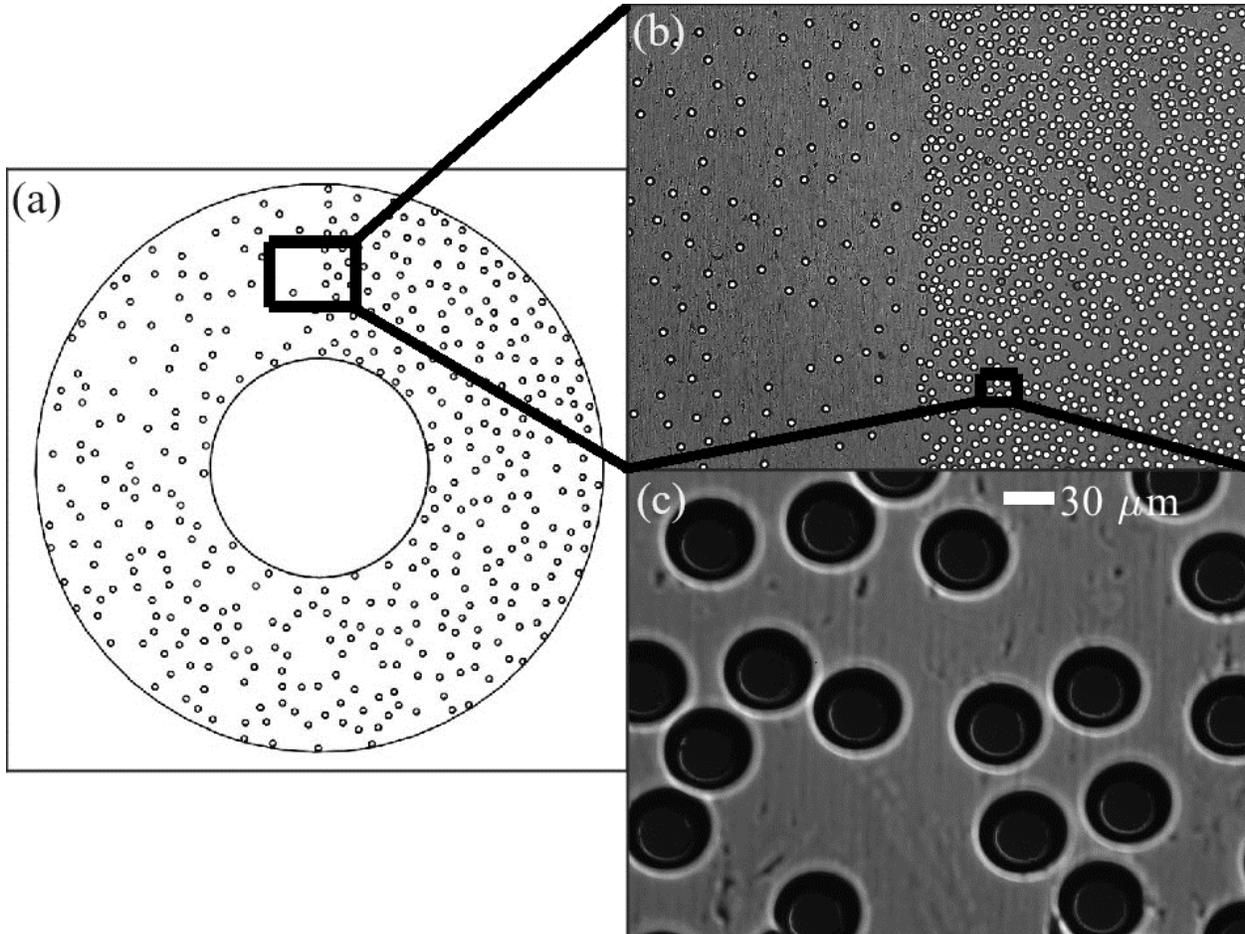
Fig. 2. Random pinhole array fabricated with a number-density gradient. (a) The simplified model of the random pinhole array. (b-c) Microscope images of the random pinhole array obtained with (b) 20x and (c) 50x magnification.
