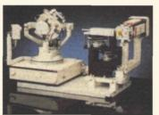
MPD1880/HR to be configured as a stand-alone system, with a dedicated X-ray tube, or as part of a multi-goniometer installation – sharing a common source with a powder, texture, or stress goniometer for complete microstructural characterization. A step size of one arc second is standard.
