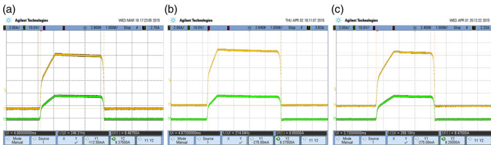
Figure 26. TCL switch resistive load response waveform: (a) ambient, (b) cold and (c) hot temperature.
