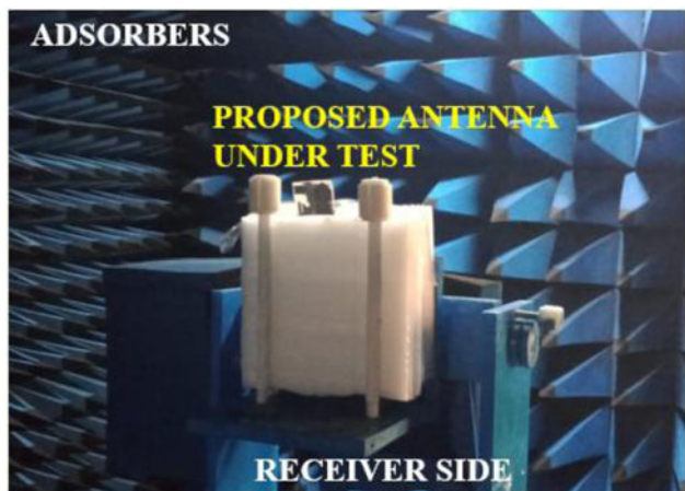
Fig. 13. Radiation pattern measurement in an anechoic chamber.
