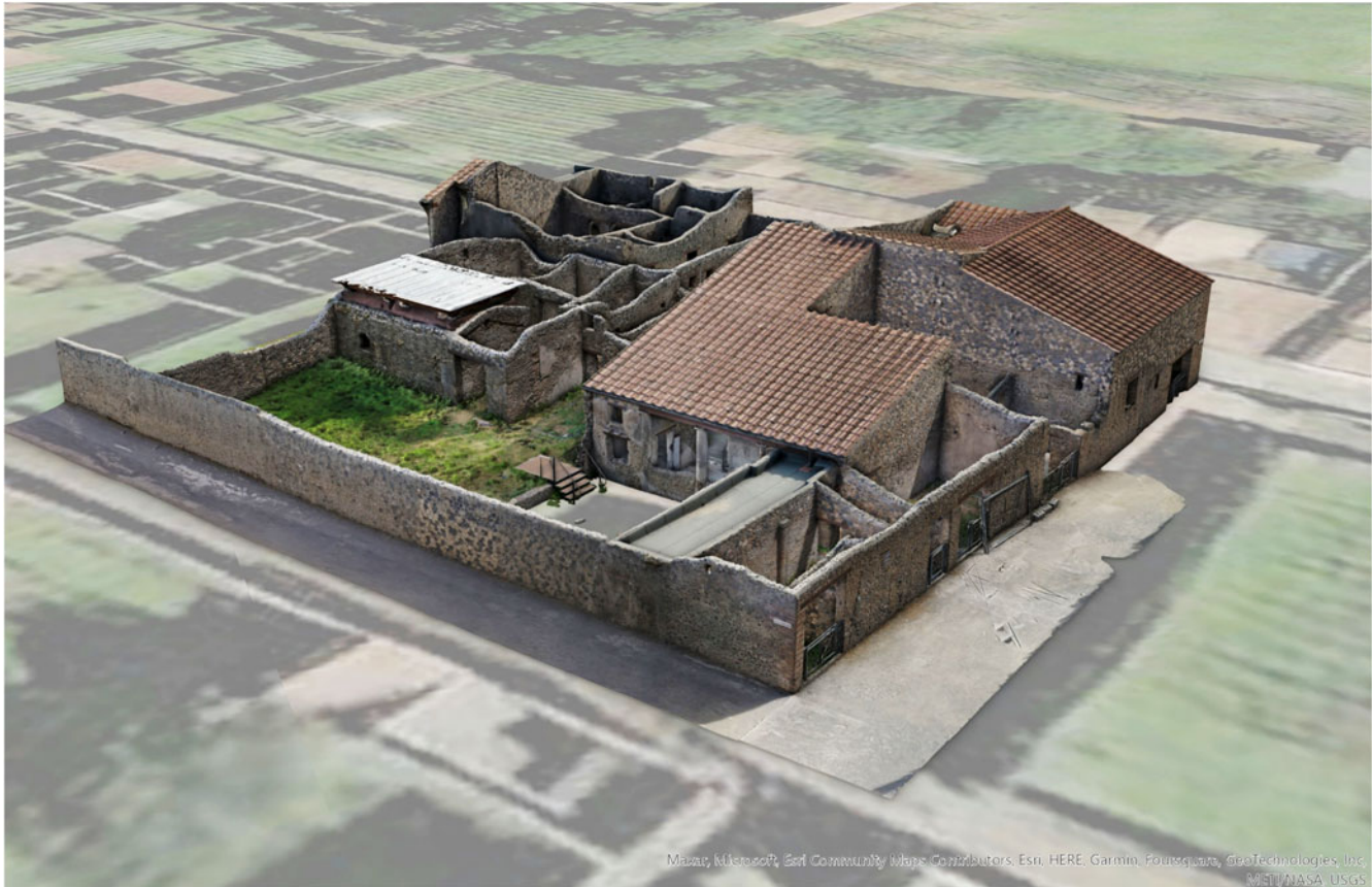
FIGURE 5. Final base model of Insula I.14. Excavation models produced during the excavation process were aligned to this referenced model.
