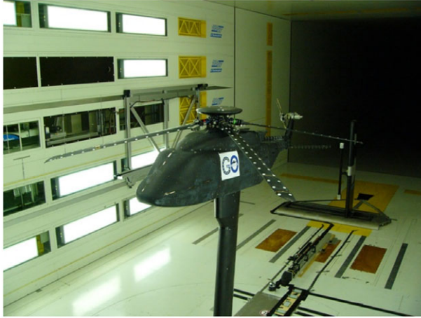
Figure 1. 7AD rotor in the GOAHEAD setup.
