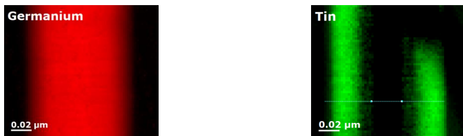
Figure 2: Elemental maps of Ge (Red) and Sn (green) obtained with EELS chemical analysis.
