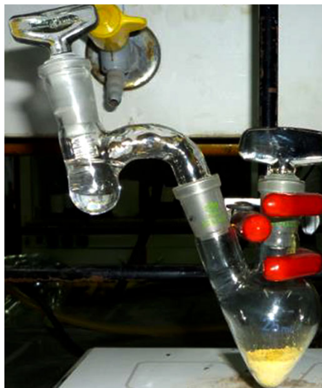
Figure 1. Air-tight polymerization flask aiming to expose the yellow-milled HNT- FeCl_3 powder to monomer vapours.
