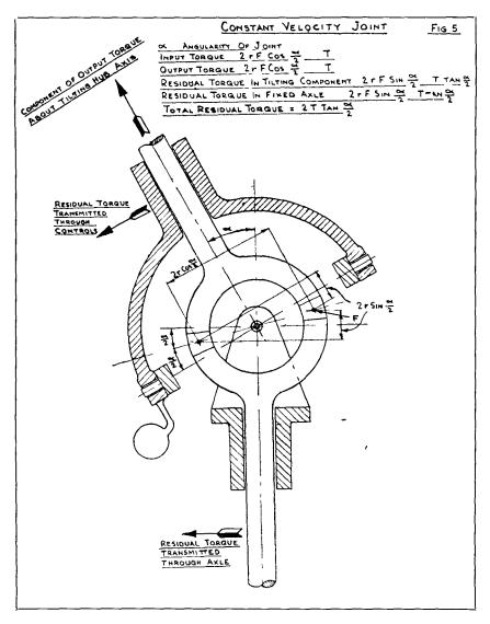
overcome the control force due to residual torque, whilst an application of control to starboard is aided by residual torque
