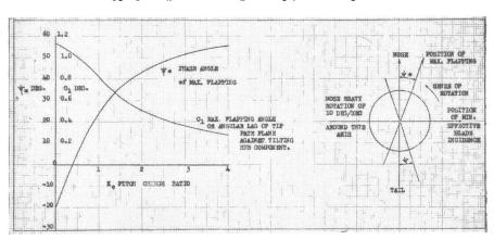
W 9 Rotor System Flapping Coefficients during 10 deg |sec Tilting Motion
