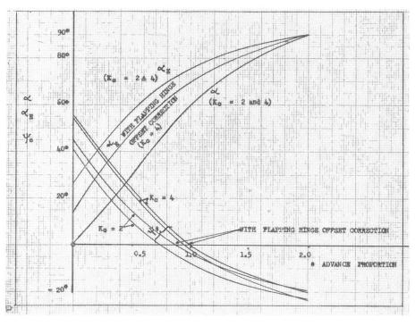
W 9 Compound Back-Coupled Rotor Relations between Functional and Geometric Parameters
