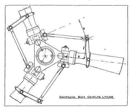
ratios are — p = g/f, q = c/f, referred to as the direct and advanced pitch change ratios These two form the coefficients in the expression for the blade pitch, where  $\theta_2$  is the representative geometric pitch of blade No 2  $\theta_0$  is the pitch setting at zero coming  $\beta_2$  the flapping angle of blade No 2,  $\beta_1$  the flapping angle of the preceding blade No 1
