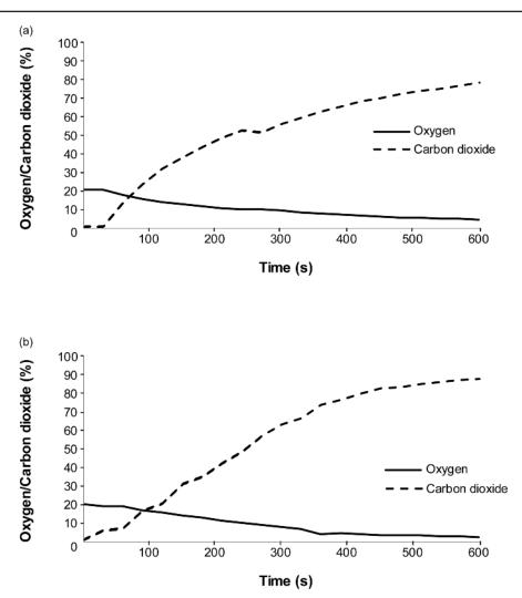
Oxygen and carbon dioxide percentages in euthanasia chamber over a 10-min period (a) when the chamber is empty and (b) when a pig is in the chamber. Time 0 is when the  $CO_2$  gas cylinder was turned on with a flow rate of 20% container volume per min.
