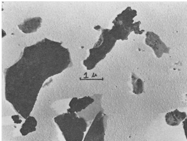
Fig. 6. Electron micrograph, 2-0.2 \mu clay fraction of A1 horizon of the somewhat poorly drained unnamed soil of the middle Coastal Plain.
