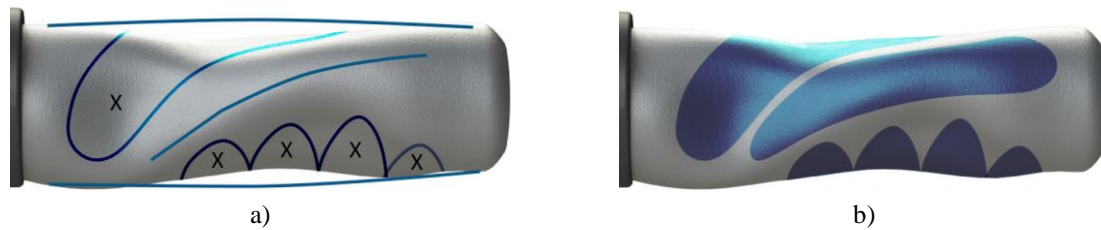
Figure 8. Layout (a) and form (b) design parameters of adaptive morphing handles
