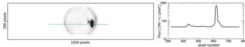
Figure 2. Simulated X-ray image of the Sun, with a C5 class flare in progress, projected on the pinhole CCD camera (left). The signal profile “observed” along the dashed line cut is shown to the right.
