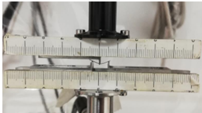
Fig.7 Three points bending test of the samples
