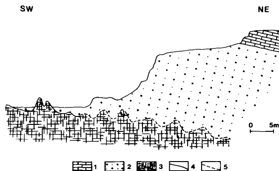
Figure 2. Vertical cross section, open pit in the Braćan deposit. 1 = hanging wall limestone; 2 = bauxite; 3 = footwall limestone; 4 = footwall boundary; 5 = tentative footwall boundary.
