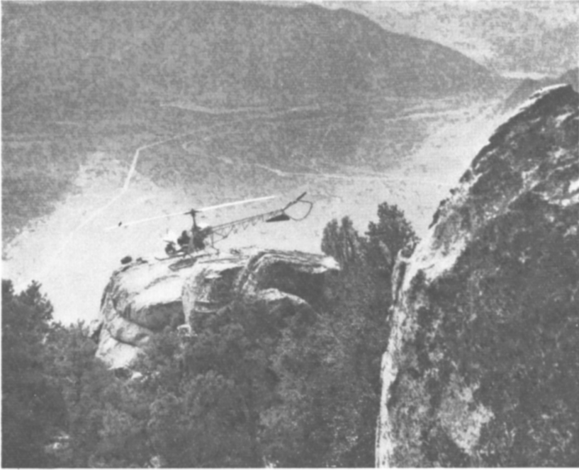
Fig 2 Showing a landing at a density altitude of 8,000 feet on a fire operation in the Sierra Mountains of California
