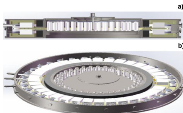
Fig. 2. Design of 0.1 Hz LTD stage with a liquid resistor load. (a) Side section view of the stage. (b) Overview of the stage.
