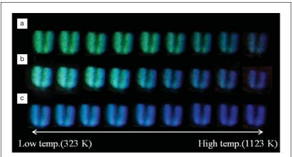
Temperature-sensitive visible photoluminescence images of Yb<sub>2</sub>O<sub>3</sub>:Tb<sup>3+</sup>/Tm<sup>3+</sup> depending on the concentration of the dopants (Tb3+ mol% / Tm3+ mol%): (a) 2/1, (b) 1/1 and (c) 0.6/1. Reproduced with permission from Opt. Lett. 36 (2011) DOI: 10.1364/OL.36.000760; p. 760. © 2011 Optical Society of America.
