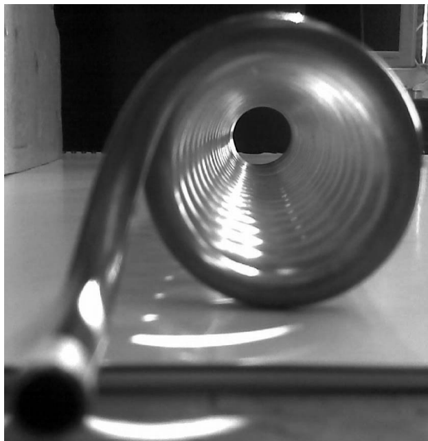
Figure 12. A standard case of LC winding. The difficulty in designing TrCs arises from the need to have smooth target travel along the LC to avoid sudden changes in the acceleration.
