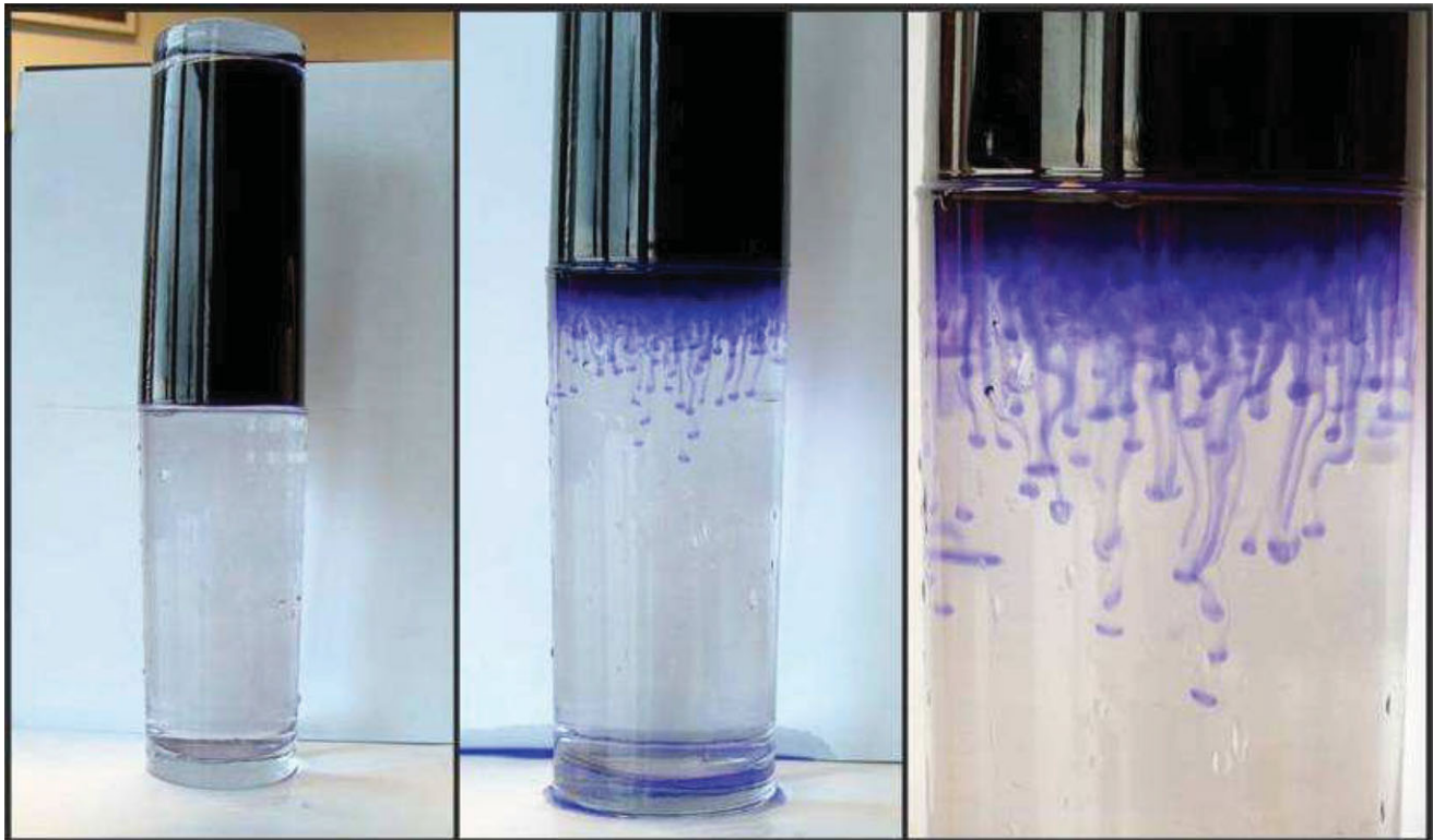
Figure 10. A simple experiment in thermohaline mixing that can be performed in the kitchen. Here some blue dye has been added to the warm, salty water to make the resulting salt fingers stand out more clearly. This experiment was performed by E. Glebbeek and R. Izzard, whom we thank for the picture.
